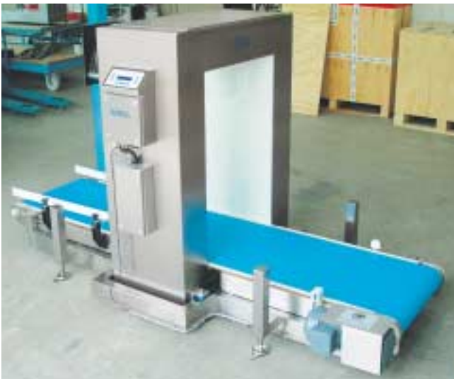
Lowrun conveyor for carton boxes
